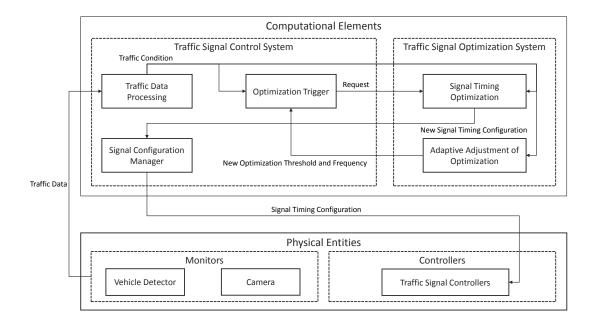
Figure 3.1: Architecture of Cyber-physical Traffic Control Systems
