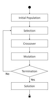
Figure 4.2: Flow chart of the genetic algorithm-based signal timing optimization
