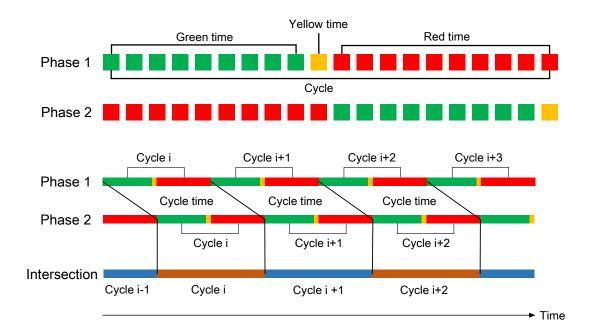
Figure 3.6: Signal timing configuration of an intersection
