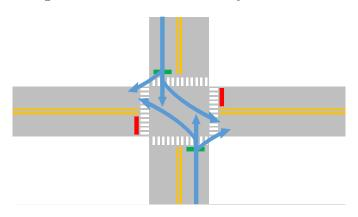
Figure 3.5: Phase 2 of four-way intersection
