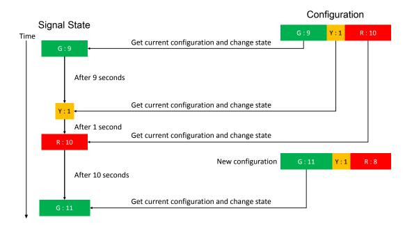
Figure 3.7: Mechanism of controller in signal display
